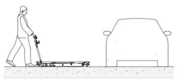
NOTE: Wheel the unit under the vehicle completely flattened down and not in the lifting position. This could cause for the lift to damage the vehicle.
