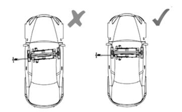
NOTE: Make sure the lift is in position underneath the vehicle straight and not at an angle. This will cause for an unstable lifting of the vehicle and could damage the vehicle. ESCO is not liable for any damage made to the vehicle due to the improper use of this lift.
