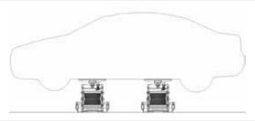
To lift the entire vehicle, use (2) miniLIFT systems. DO NOT attempt to lift vehicle using only (1) miniLIFT. This could result in damage to the vehicle or even worse serious injury or death.
