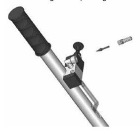
Install Air Nipple (1/4 INCH NPT) into handle using teflon tape (or equivalent). Properly tighten air nipple onto the handle and test for any leakes in the connection and/or the air hose. DO NOT operate miniLIFT with damaged or leaking air hose and/or input nipple.
