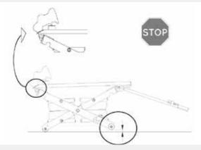
NOTE: If at any time the back wheels of the miniLIFT begin to lift off of the ground while the lift is in use STOP IMME-DIATELY. Slowly release the air from the miniLIFT until the wheels are back on the ground safely. REMINDER: miniLIFT must lift on a solid flat foundation.
