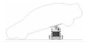
miniLIFT can lift the vehicle from one end or the other. the minilift is NOT a full vehicle lift system on its own.
